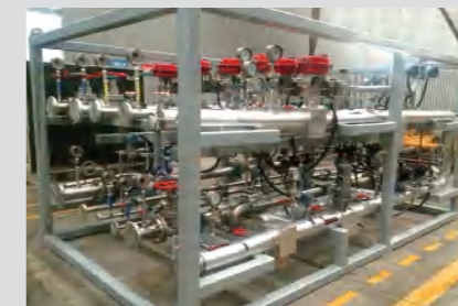
氧气、天然气、重油混合撬 Gas Mixing Skid of O2 & NG & Heavy Oil
